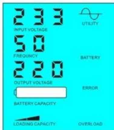
Battery dead, utility supply power
