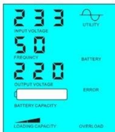
Battery dead, utility supply power
