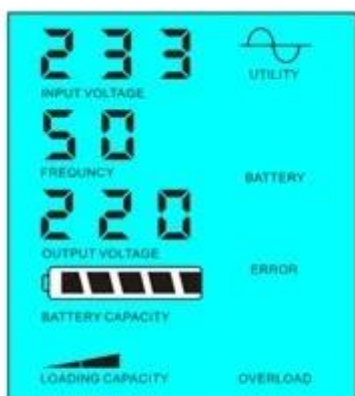
Utility supply power and charge battery
