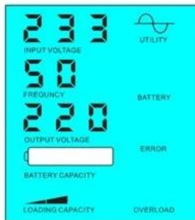
Battery dead, utility supply power
