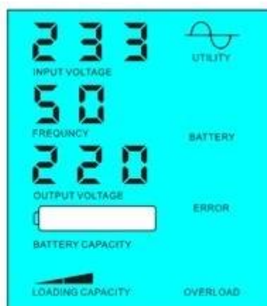
Battery dead, utility supply power
