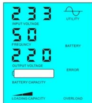
Battery unavailable, utility supply power
