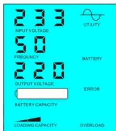
Battery unavailable, utility supply power
