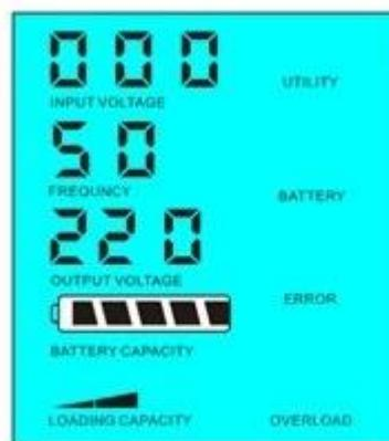
Load's power > 5% of inverter's rated power
