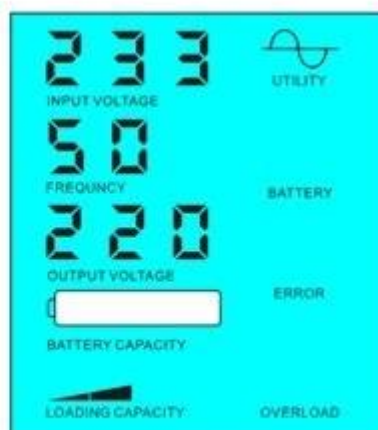
Battery dead, utility supply power
