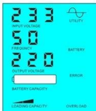
Battery dead, utility supply power
