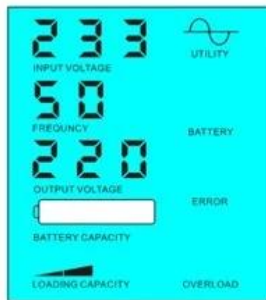
Battery dead, utility supply power
