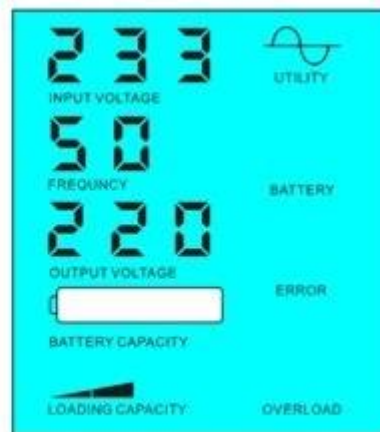
Battery dead, utility supply power
