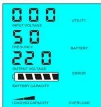
Load's power > 5% of inverter's rated power
