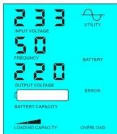
Battery dead, utility supply power
