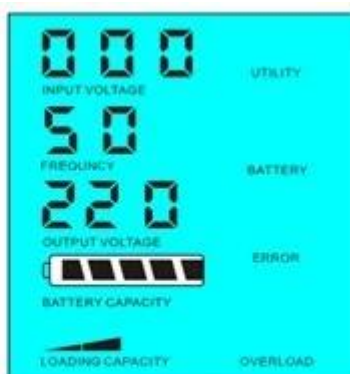
Load's power > 5% of inverter's rated power
