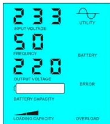
Battery unavailable, utility supply power
