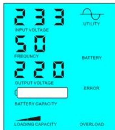
Battery unavailable, utility supply power
