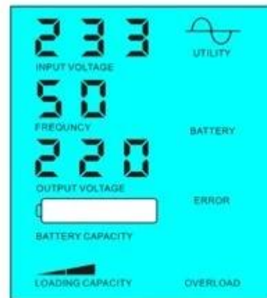
Battery dead, utility supply power
