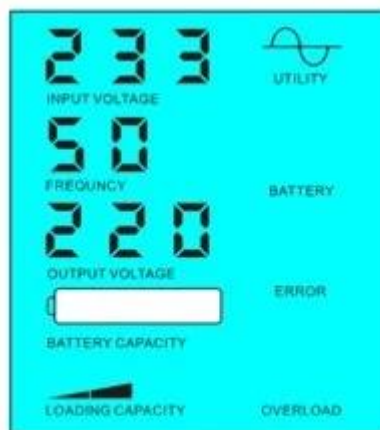
Battery dead, utility supply power
