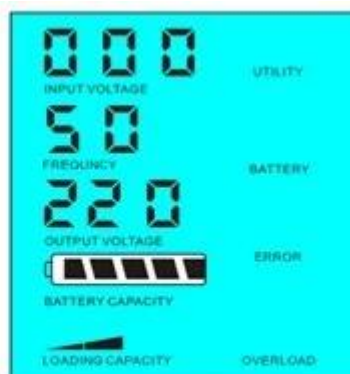
Load's power > 5% of inverter's rated power
