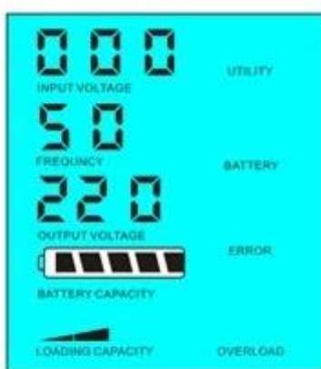
Load's power > 5% of inverter's rated power
