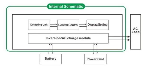
Utility first battery standby UPS mode (on the panel turn the button to "AC")
