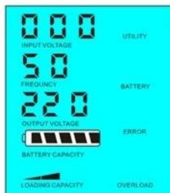
Load's power > 5% of inverter's rated power
