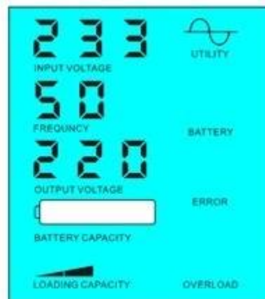
Battery dead, utility supply power
