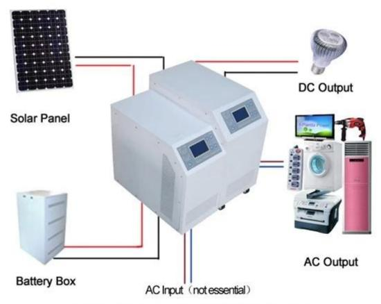
I-P-HPC-Series Inverter+MPPT Solar Controller
