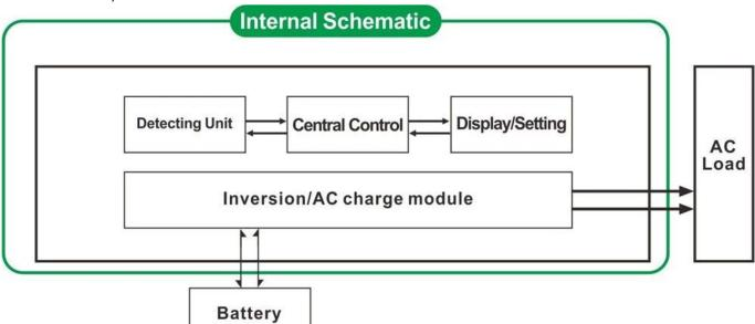
1.1 Normal working mode (ON): No matter it's connected AC loads or not
