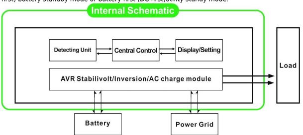
2.1 Utility first (AC first) battery standby mode : FREQUENCY in the LCD display is set to 01. When utility
