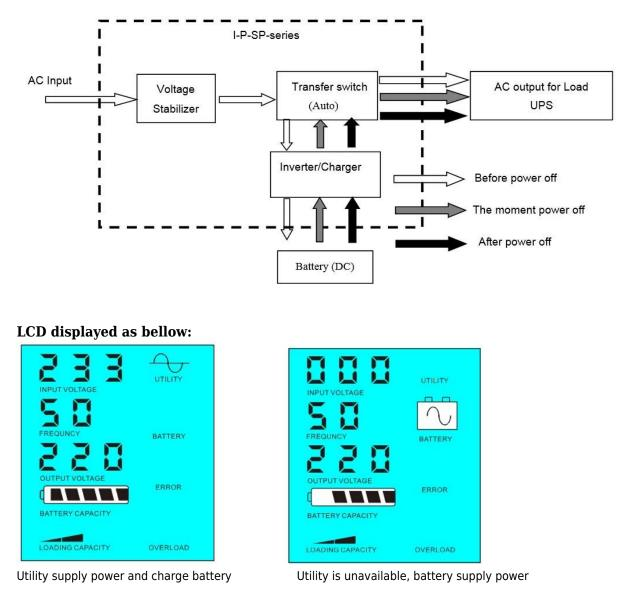
2.2 Battery first (DC first)utility standby UPS mode: FREQUENCY in the LCD display is set as 03. When utility and battery are connected to the inverter, battery will supply power to the loads prior to utility. When battery capacity is not enough, utility will continue to supply power automatically.
