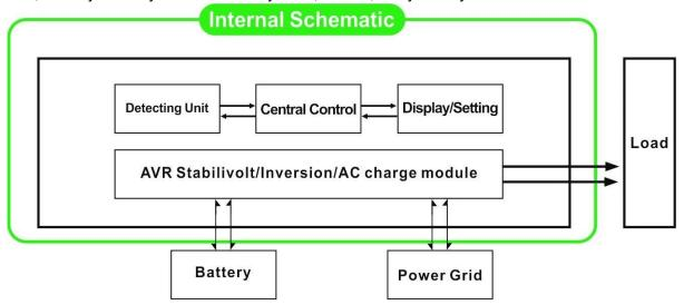
2.1 Utility first (AC first) battery standby mode: FREQUENCY in the LCD display is set to 01. When utility and battery are connected to the inverter, utility will supply power to the loads prior. When utility is cut off,
