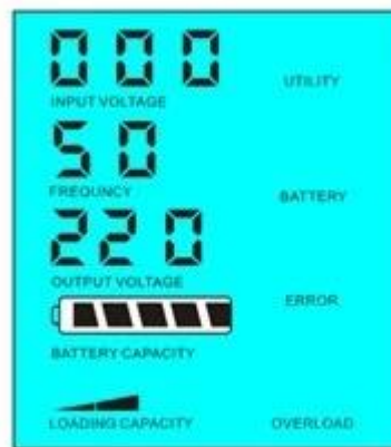
Load's power > 5% of inverter's rated power
