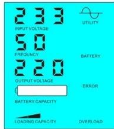
Battery dead, utility supply power
