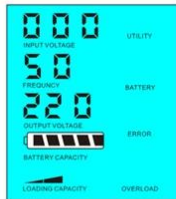
Load's power > 5% of inverter's rated power
