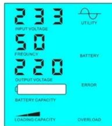
Battery dead, utility supply power
