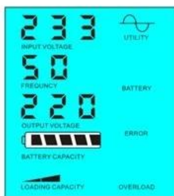
Utility supply power and charge battery
