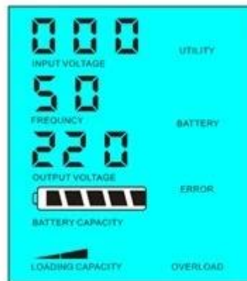
Load's power > 5% of inverter's rated power
