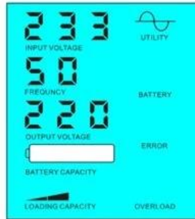
Battery dead, utility supply power
