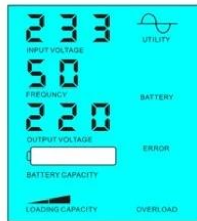
Battery dead, utility supply power
