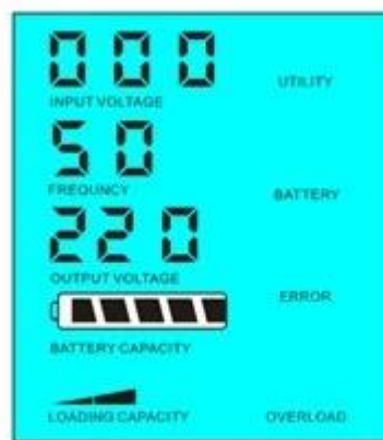
Load's power > 5% of inverter's rated power
