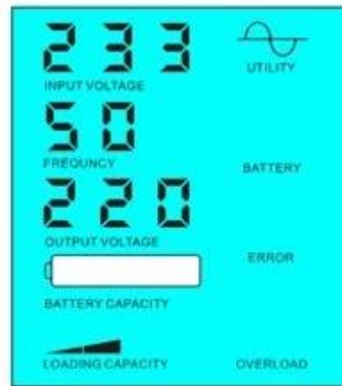
Battery dead, utility supply power
