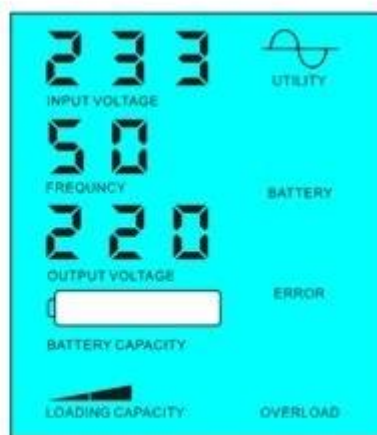
Battery dead, utility supply power
