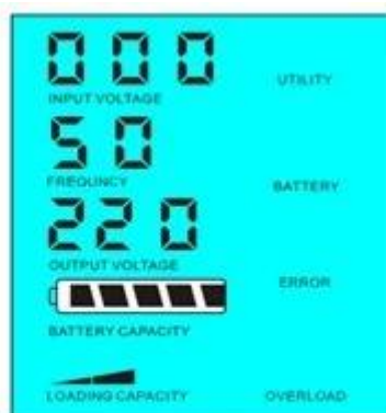
Load's power > 5% of inverter's rated power
