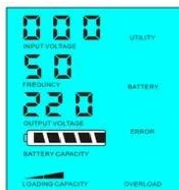
Load's power > 5% of inverter's rated power
