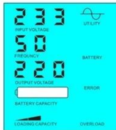
Battery dead, utility supply power
