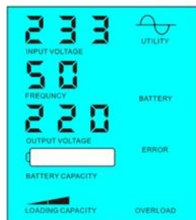
Battery unavailable, utility supply power
