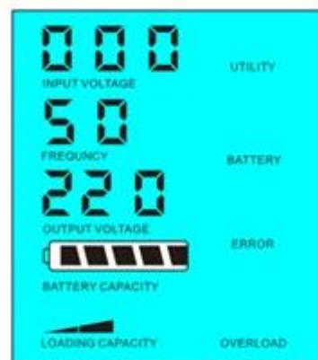
Load's power > 5% of inverter's rated power
