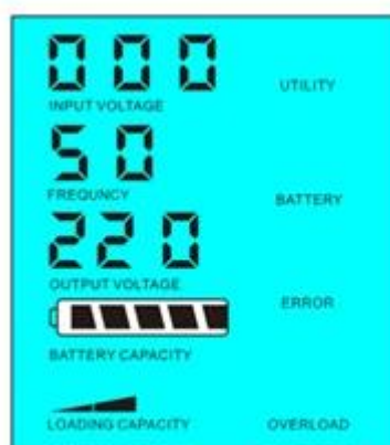
Load's power > 5% of inverter's rated power
