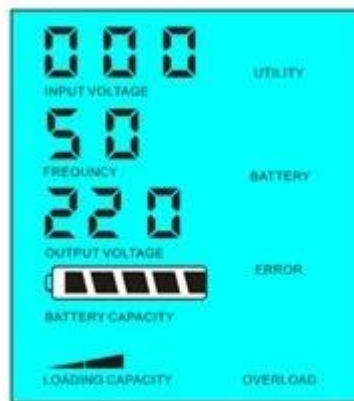
Load's power > 5% of inverter's rated power
