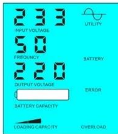
Battery dead, utility supply power
