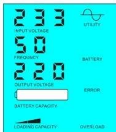
Battery dead, utility supply power
