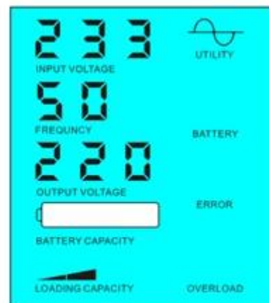
Battery unavailable, utility supply power
