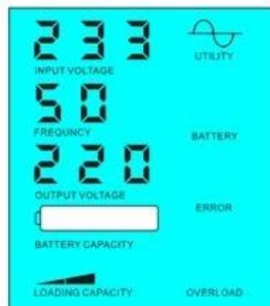
Battery dead, utility supply power
