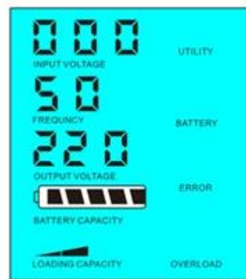
Load's power > 5% of inverter's rated power
