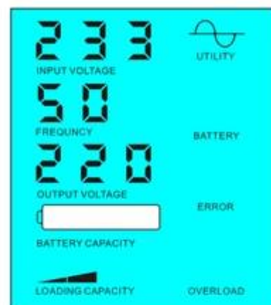
Battery unavailable, utility supply power
