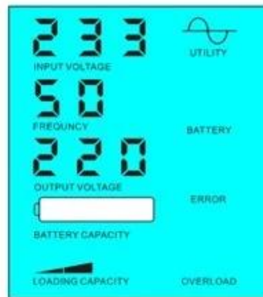
Battery dead, utility supply power
