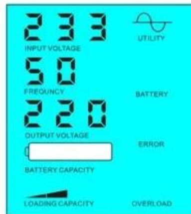
Battery dead, utility supply power
