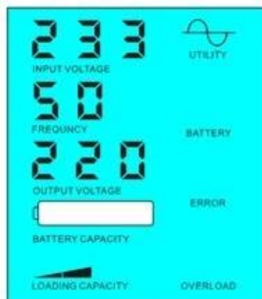
Battery dead, utility supply power
