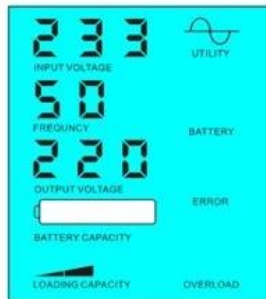
Battery dead, utility supply power
