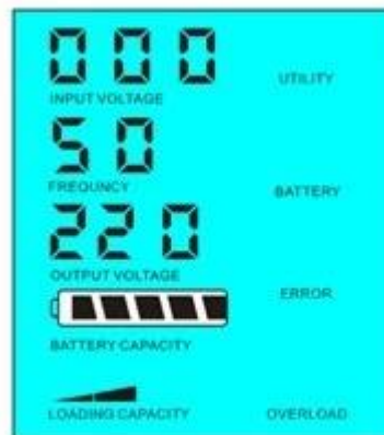
Load's power > 5% of inverter's rated power
