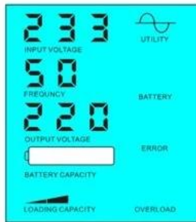
Battery dead, utility supply power
